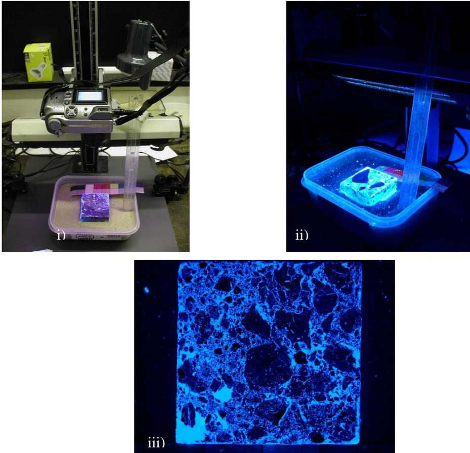
Figure 2.2: Images show Ultra Violet imaging of resin impregnated soil blocks. i) Copy stand, camera and UV light source set-up. ii) Florescent soil block surface. iii) Example of good impregnation and imaging of soil surface.
