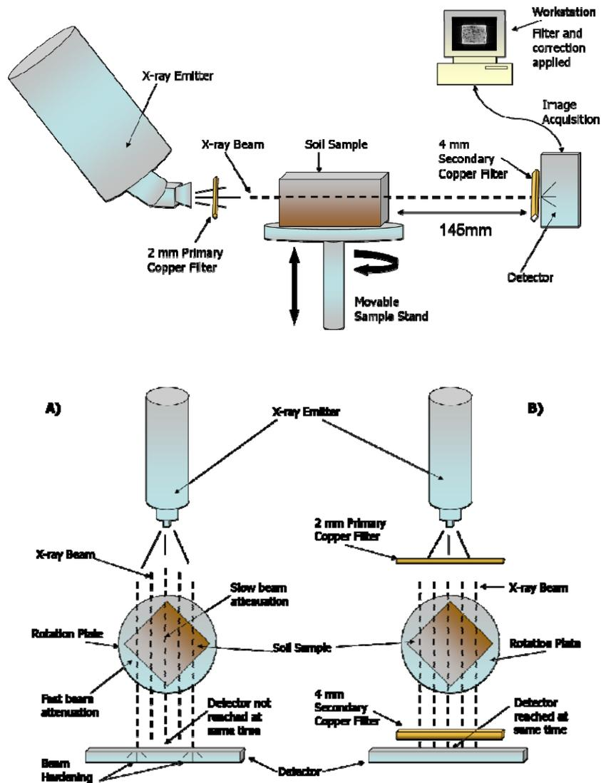
Figure 2.1: X-ray computed tomography diagram of set-up and the effect of beam hardening (a) due to faster x-ray and the correction applied using copper filters (b) in preventing beam hardening.
