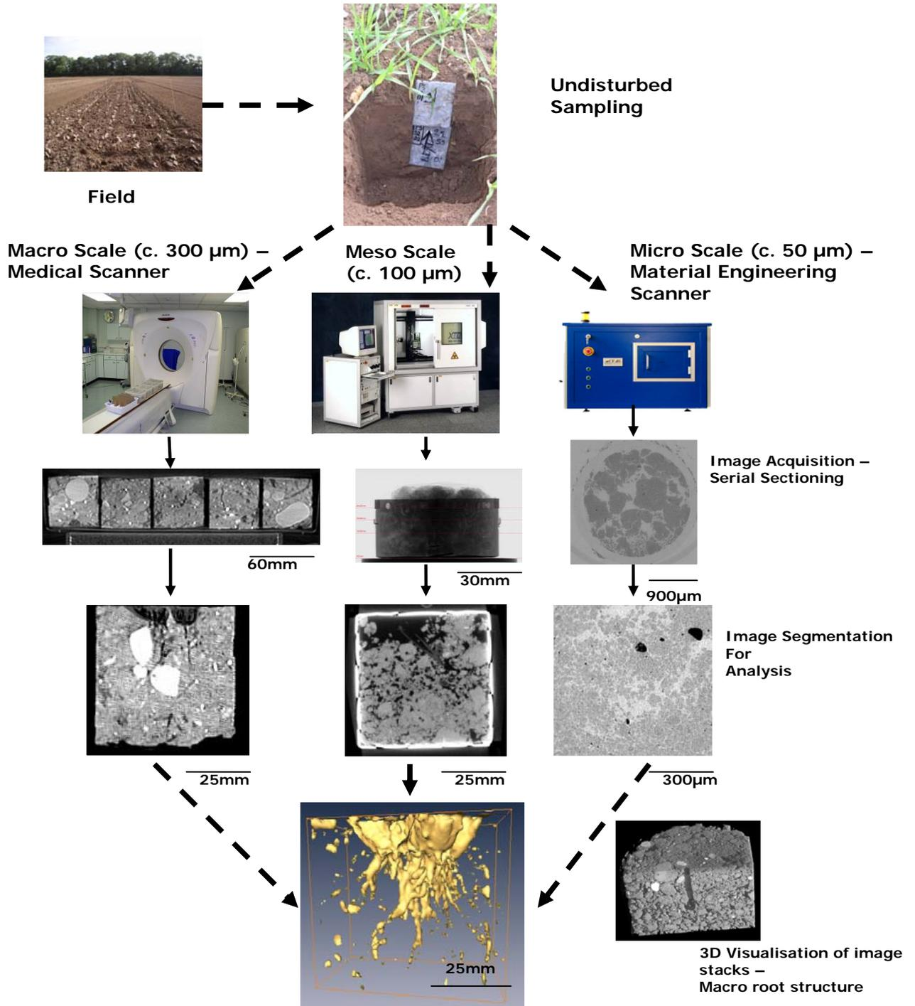
Figure 1.3: X-ray Computed Tomography scales of resolution and image acquisition through to analysis and 3D visualisation applications for quantifying soil structure.
